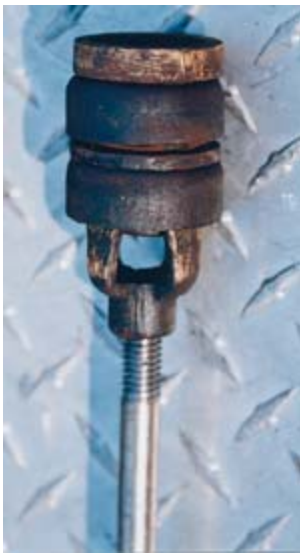
Close-up of leather seals on plunger
