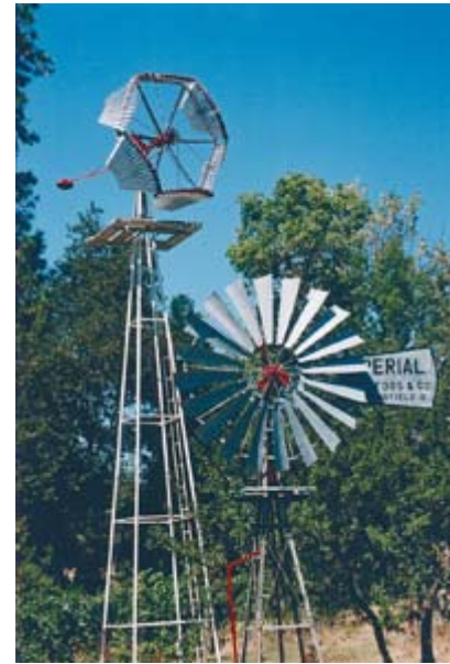
The windmill on the left is a Baker Monitor "vaneless" (no tail) with "football" counterweight. Folding wheel opens and closes the hole in the middle to regulate the speed.
