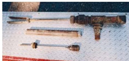
From top to bottom: Pump-rod assembly, cylinder, and plunger with leathers
